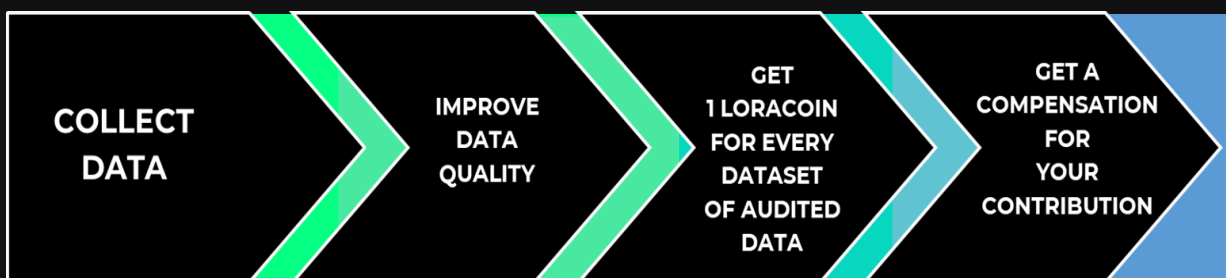
Fig.7: LoRaTRUST process IoT data delivering feedback on data quality, and compensating the user according to the amount of quality data collected.
